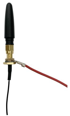
If a good ground plane is not available, a radial ground plane can be applied as the picture. The wire size is 1/4 wavelength referred to the working frequency of the antenna, connected to ground, as close as antenna connector. See picture above.
